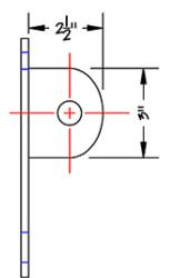
The female has two  $\frac{1}{2}$ " tabs with holes that will fit a  $\frac{3}{4}$ " bolt or pin, and would be used on an 8" Truss Frame.
