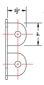
The female has four  $\frac{1}{2}$ " tabs with holes that will fit a  $\frac{3}{4}$ " bolt or pin, and would be used on an 8" Truss Frame.
