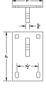
The male has one  $\frac{5}{8}$ " tab with a hole that will fit a  $\frac{3}{4}$ " bolt or pin, and would be used on an 8" Truss Frame.
