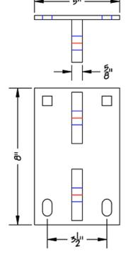
The male has two  $\frac{5}{8}$ <sup>11</sup> tabs with holes that will fit a  $\frac{3}{4}$ <sup>11</sup> bolt or pin, and would be used on an 8<sup>11</sup> Truss Frame.
