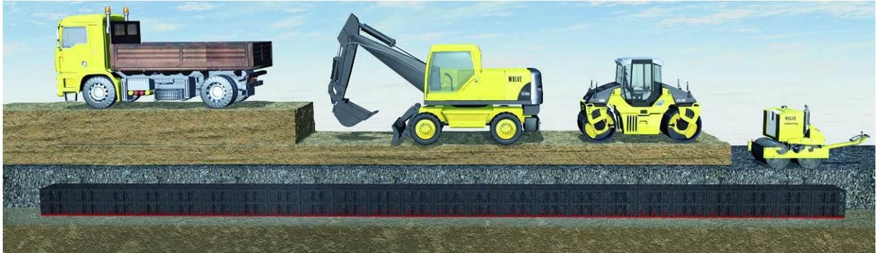
Various construction machinery may be used to fill the excavation. Given the additional dynamic loads they cause, compression equipment must not be driven directly over the EcoBloc Inspect system and compression equipment with activated vibration motors must not be taken over the area.
