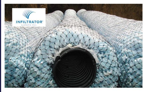
Manufactured from recycled materials, these lightweight EZ Flow Drainfield Systems come in bundles that can be hand-carried into position, making them quick to install and saving costs on heavy machinery and labour. Their modular construction allows configurations to match trench dimensions for most system shapes and sizes. Their flexible design gives them the ability to contour along sloped sites and around trees or landscaping.
